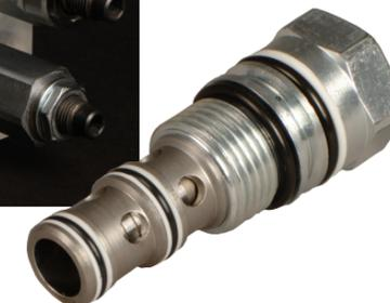
This space-saving manifold uses two multi-function valves. The ventable FR valve (located in the top of the manifold and pictured below it) sends priority flow to an accumulator that, once charged, assures adequate pressure at all times for the brakes. Once the accumulator is charged, the UPCV valve (pictured at left) automatically unloads the pressure to make it available for other machine functions.
