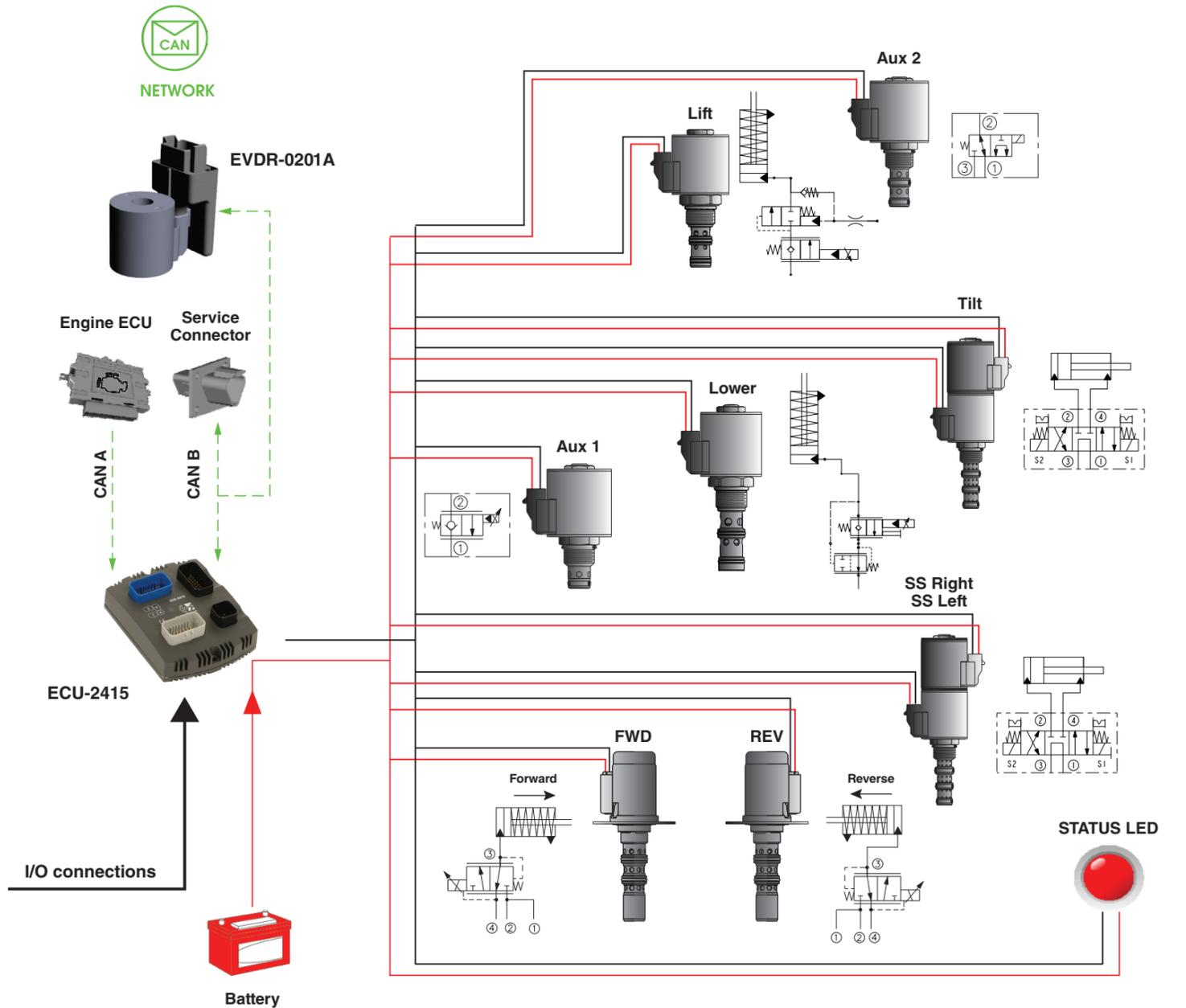
This diagram depicts a fully integrated electrohydraulic control system. Inputs and outputs are controlled by a single ECU-2415.
