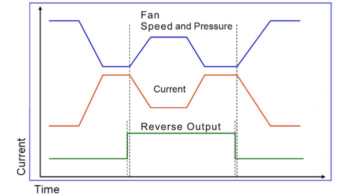
Control valves with multiple temperature inputs can be used to provide variable fan speed control depending on air temperature, load and cooling requirements. If the radiator gets clogged, the electro-proportional valves can automatically reverse fan direction.
