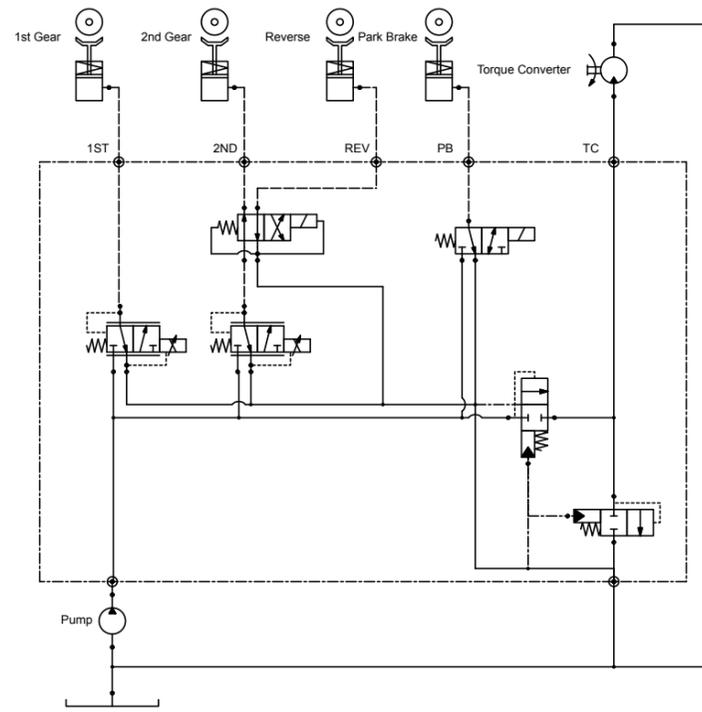
A typical two-speed transmission for a telehandler
