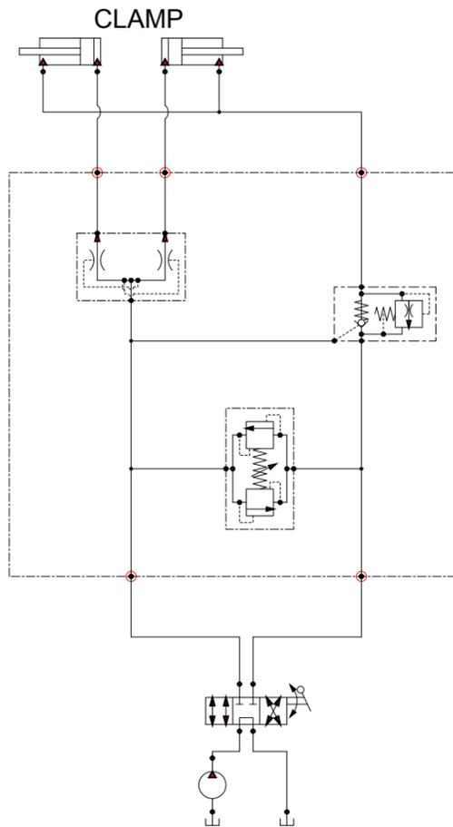
This circuit shows how you can control a carton clamp attachment. It uses a flow divider combiner to maintain equal pressure on both arms of the clamp.
