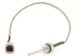
The HydraForce ERT120 sensor is designed for use in demanding industrial applications. It can sense temperatures from -40 to 150° C (-40 to 300°F) and has a padded resistor for improved linearity of the input curve.
