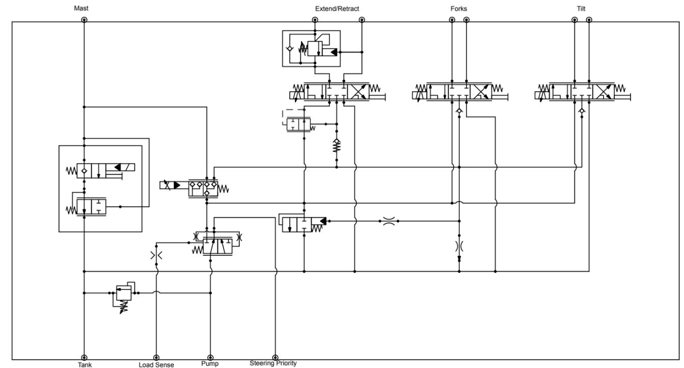
This circuit for a three-wheel electric counterbalance truck uses the force of gravity for lowering rather than hydraulic pump pressure, which saves energy and fuel. A previous manifold required pilot pressure to activate the lower spool.
