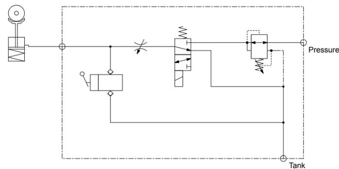
This circuit uses a solenoid valve to provide hydraulic pressure to power off the brake, a needle valve to control how quickly the brake is applied and released, and a hand pump to allow emergency braking.
